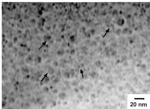
Figure 7. TEM showing the clustering of several smaller sized CdTe nanocrystals, more clearly shown in a few CdTe growth islands marked by arrows. The islands have an average size \sim 15 nm and are dispersed in the \text{TiO}_2 matrix for a 1500 Å thick film deposited at T_s = 27^\circ\text{C} .
